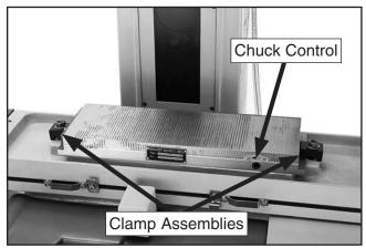
Figure 23. Magnetic chuck attached to table.
